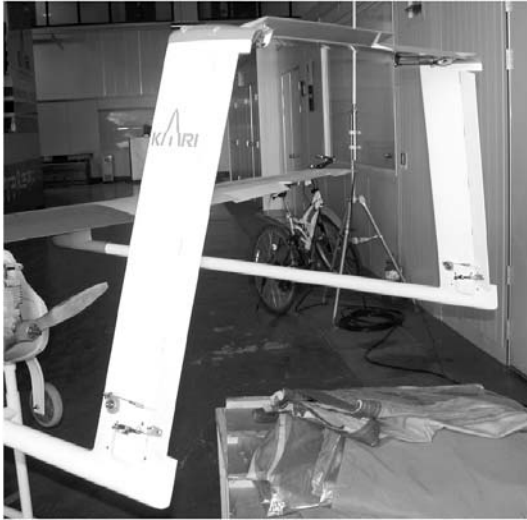
Fig. 2 Split in elevator and addition in rudder
